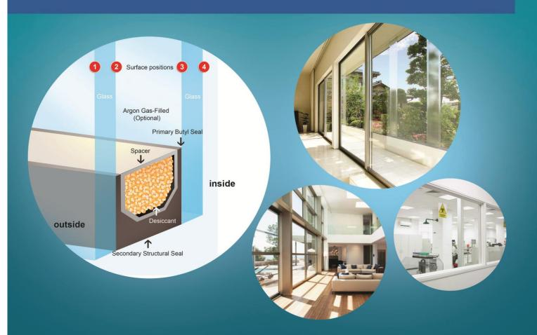
ThermaPro® Insulated Glass Units are manufactured on a made-to-order basis. Glass panes are cut to size and washed for optimum clarity while air spacers of specified thicknesses are cut and assembled into the required overall dimensions. An adhesive sealant holds the spacer and glass together. Each unit is then sealed on the edges using structural silicone sealant to prevent humid air from entering the units, guaranteeing a clear view any time of the year.
